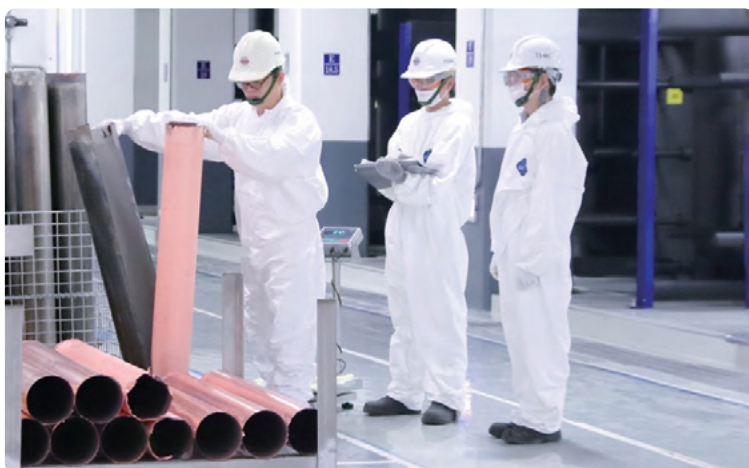
TSMC recycles waste cupric sulfate that was originally outsourced for treatment into copper tubes.
